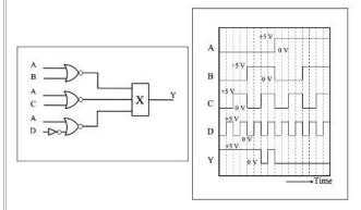
To obtain the output Y as shown in the figure, the logic gate X should be
